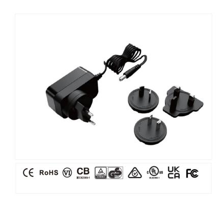
The 56YSV12-xy-RS Series is a regulated and reliable 12W Interchangeable AC/DC Plugtop Adapter Power Supply. Designed for use in applications such as system-critical media and control infrastructure. This series is supplied with a Interchangeable input connection and supports input voltages of 90~264V AC 50~60Hz.
